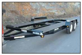
MODEL CH16-7-FULL CH18-7-FULL CH18-10-FULL 82"x16' 82"x18' **BED SIZE** 82"x18' **GVWR** 7.000 LBS 7,000 LBS 10.000 LBS **EMPTY WT** 1.990 LBS 2.105 LBS 2.255 LBS **DECK HEIGHT** 20" 20" 20" ST205/75R15C ST205/75R15C ST225/75R15D TIRES AXLE 3.500 LBS (2) 3.500 LBS (2) 5,200 LBS (2) COUPLER 2 5/16" A Frame 2 5/16" A Frame 25/16" A Frame JACK 5.000 LBS Top Wind 5,000 LBS Top Wind 5.000 LBS Top Wind
