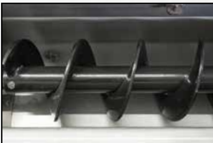
Heavy Duty 9 inch Dia. Auger for 92450SSA 6 inch Dia. Auger for all other models
