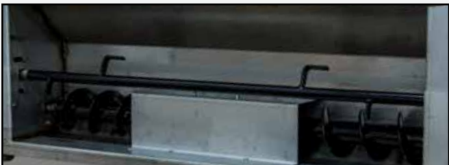
5" Dia. Auger and mixing tines *(5535000)
