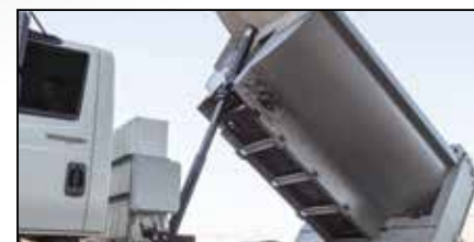
Mailhot® multi-stage, double-acting, nitrided cylinder, trunnion-mounted hoist
