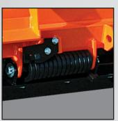
Trip Edge Features: Multi-Section 1/2" steel trip edge for independent tripping to maximize ground clearing. 3/4" square steel torsion trip springs for maximum strength. Preloaded brackets keep springs under tension. 1/4" diameter pins
