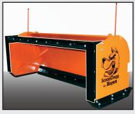
The back drag kits include a 1" x 6" rubber cutting edge mounted to a black powder coat steel frame & a set of 3/4" thick abrasion resistant steel wear shoes. The edge is mounted to the top of the ScoopDogg<sup>™</sup> & the shoes are mounted to the front of the side plates. When mounted, and with the ScoopDogg rotated forward, the back drag kit can be used to pull snow away from buildings, docks and other tight places. The kit is bolt-on & removable.
