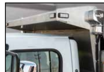
Cab shield with Built-In Tarp System
