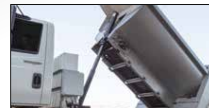
Mailhot® multi-stage, double-acting, nitrided cylinder, trunnion-mounted hoist
