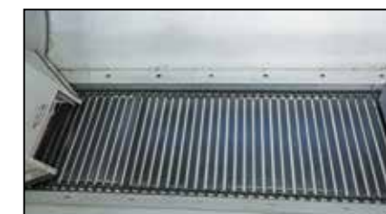
30.25" wide conveyor with 1/2" bars
