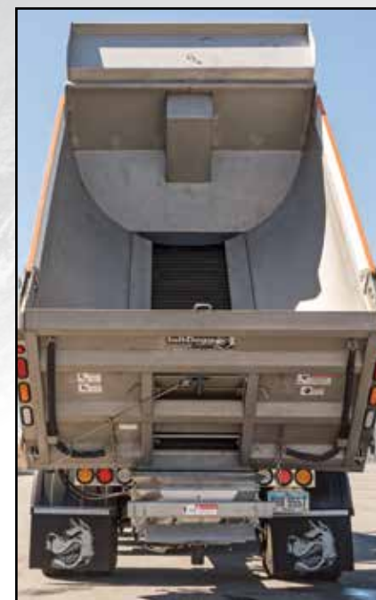
Unique, roll-formed sides and cross member-less design
