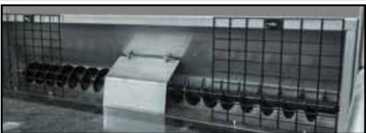
6" dia. auger and screen
