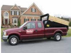
TC - 101 MAGNUM - Our steel pickup insert w/telescopic cylinder. Dumps 6,200 lbs., And has 2.5 cu. yd. cap.; Weighs just 600 lbs. Models for 8 ft. or 6.5 ft. pickups. Pre-assembled unit installs quickly with just two bolts.
