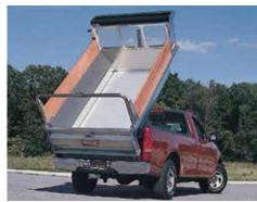
TC - 121 ULTRA - An all aluminum and stainless steel unit; 7000 lb. and 2.4 cu. yd capacity; Adds approx. 400 lbs. to your truck; For full size pickups; Virtually no maintenance; Greater payloads and hauling volume. Shortbed model available.
