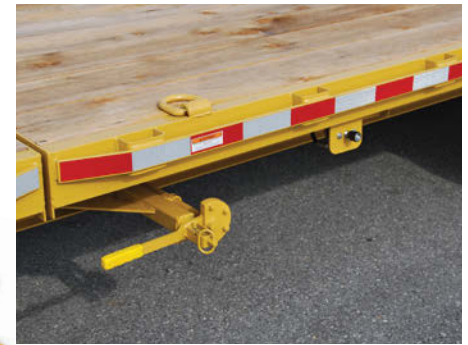
Adjustable Cushion Cylinders & Locking Mechanism
