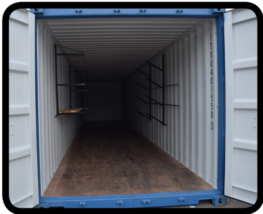
Inside View, with Pipe Racks
