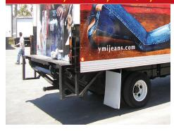
The two standard oversized platforms offer increased productivity at a budget price level. Platform sizes up to a length of 48" offer the best of both worlds with decreased platform angle, more space in front of cart stops and easy access on and off the platform.
