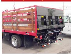
Streamlined cantilever gate with simplified controls. Multi-purpose unit designed for medium duty weight applications. Ideally suited for lower bed heights. Works well with various rear door configurations.
