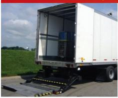
ILFP combines a column lift type, large flat platform with the un-obstructed dock loading access of an under slider. This lift works with most door configurations and is available for both trailers and straight trucks.
