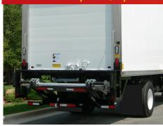
Twin cylinder liftgate designed for walk ramp dual purpose applications. Heavy duty construction with aluminum platform, slide in PowerPack and standard three piece rear impact guard.
