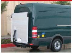
External mounted solution for panel van applications. Bolt on installation prepared for each model (specify with lift order). The MiniFix does not accommodate the optional Sprinter step bumper. The spare tire has to be relocated from under the vehicle.
