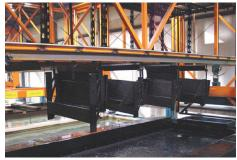
Once painted, the liftgate is rinsed to recycle any un-deposited paint, achieving nearly 100% paint efficiency for an environmentally friendly process.
