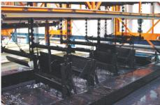
The liftgate is fully immersed in a PPG paint bath where direct current is applied between the steel and counter electrodes. Paint is attracted by an electric field to the lift gate until every bare steel part is covered and the field is broken.
