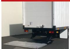
The ILU is a rapid mount, value added and streamlined under slider stored under the vehicle in a protected position ready for dock loading without any additional operations.
