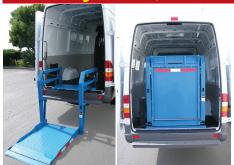
Internal mounted solution for panel van applications. The CityFix is a fast and easy bolt on installation which accommodates the different bumpers on the Sprinter. The spare tire can stay in place. Longer platforms require more interior height in the truck.
