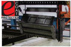
PALFINGER Liftgates are cleaned in a series of four baths, then pre-treated with a phosphate conversion coating to prepare the liftgate for electro coating.
