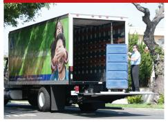
Offers a large capacity level ride platform and is stored under the vehicle in a protected position ready for dock loading without any additional operations. Stores out of the way, use only when needed.
