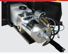
Production of PALFINGER liftgates start with using the best available components designed for years of hard labor. PALFINGER products feature heavy duty, hardened and corrosion protected pins with low maintenance greasable bushings. The power packs are equipped with thermo switch protected motors and extra heavy duty motor solenoids.
